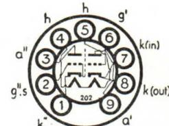
The BRIMAR PCC84 consists of two separate high slope triode units designed for use in VHF cascode amplifiers. Normally, triode 1 is operated as a grounded cathode stage directly coupled to triode 2 which is connected as a grounded grid stage. This gives a low noise input amplifier for use in television receivers for Band III. The shield connected to the grid of triode 2 keeps coupling between the two units to a minimum.
