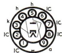
The BRIMAR Type UY85 is a half-wave rectifier for use in A.C./D.C. receivers where a 0.1 amp. series heater chain is employed.
