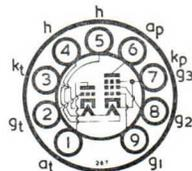
The BRIMAR UCL83 is a triode and output pentode with separate cathodes designed primarily for use in A.F. applications.
