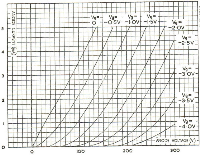
CHARACTERISTIC CURVES: g_m/V_g — Triode Section
