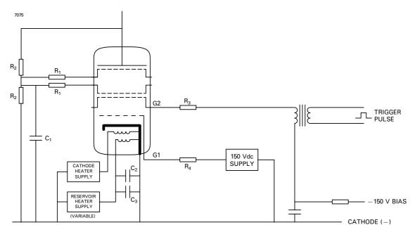
$R_1 = 470 \Omega 12 W$  vitreous enamelled wirewound resistors.
