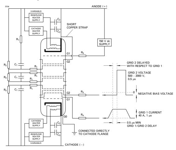
$R_1 = 470 \Omega 12 W$  vitreous enamelled wirewound resistors.
