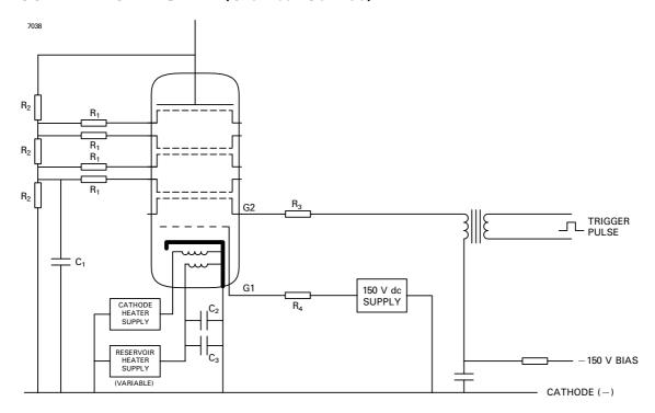
$R_1 = 470 \Omega$  12 W vitreous enamelled wirewound resistors.
