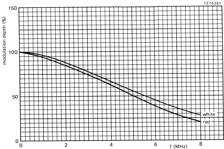
Fig.4 Typical square-wave modulation transfer characteristic.
