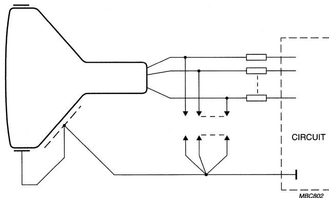
Fig.15 Flashover protection circuit.
