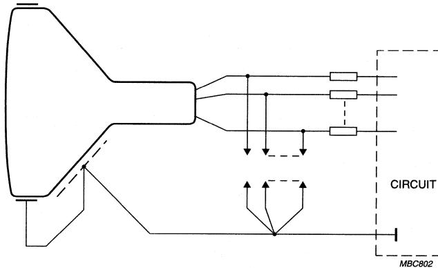
Fig.14 Flashover protection circuit.
