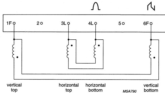
Fig.4 Electrical diagram of deflection coils.
