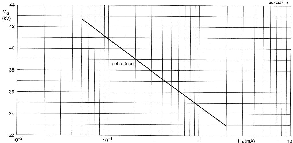
Fig.16 0.5 mR/h iso-exposure-rate limit curve.
