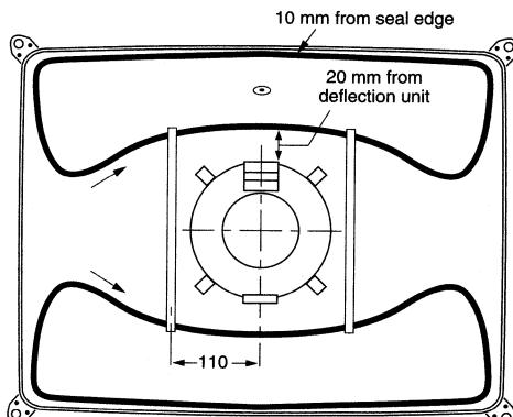
Fig.20 Position of double degaussing coils on the picture tube.
