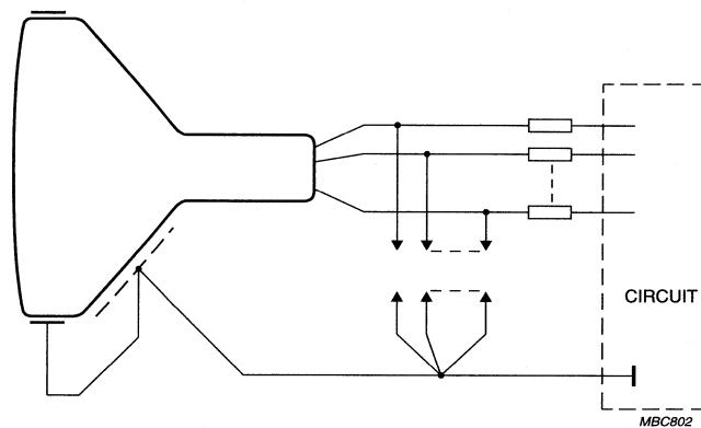
Fig.13 Flashover protection circuit.
