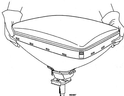
Fig.21 Lifting tube from face-up position.
