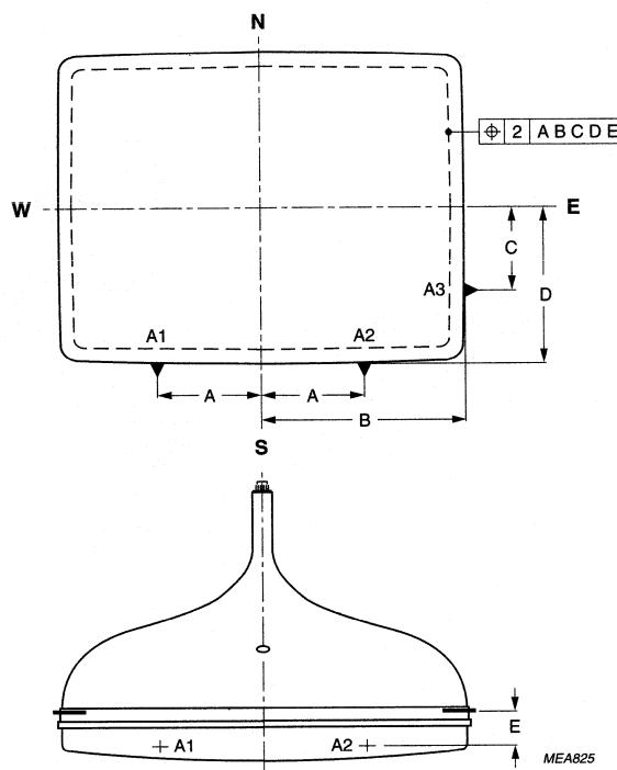
Fig.1 Phosphor alignment.
