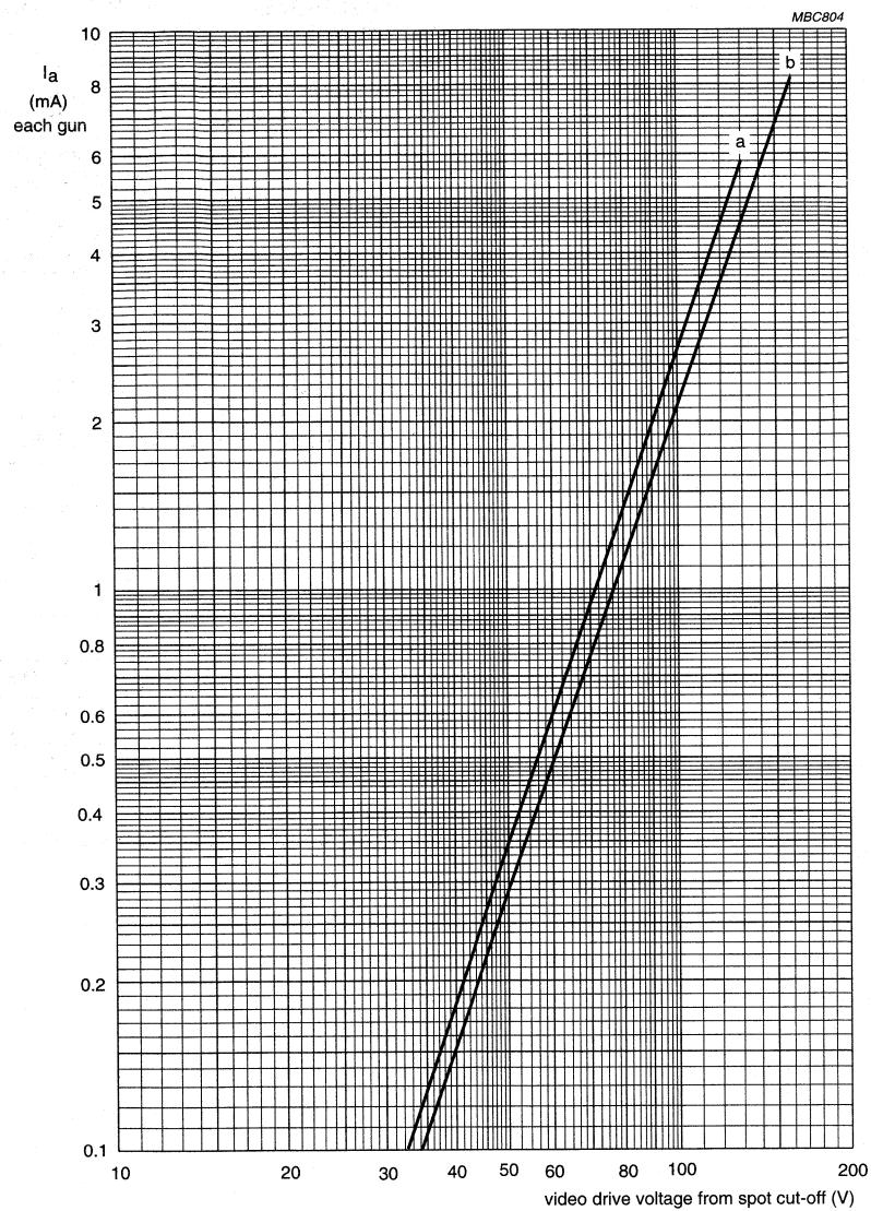
$V_f = 6.15 \text{ V}$ . $V_{a,g4} = 27.5 \text{ kV}$ . $V_{g3}$  adjusted for focus.V<sub>g2</sub> (each gun) adjusted to provide spot cut-off for  $V_k = 130 \text{ V}$  (curve a) and  $V_k = 160 \text{ V}$  (curve b).
