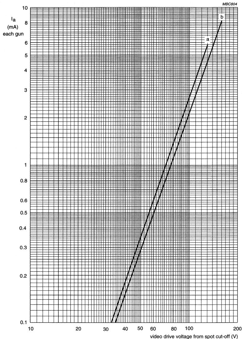
$V_f = 6.15$  V. $V_a = 27.5$  kV. $V_{g3}$  adjusted for focus. $V_{g2}$  (each gun) adjusted to provide spot cut-off for  $V_k = 130$  V (curve a) and  $V_k = 160$  V (curve b).
