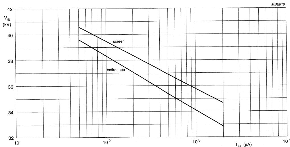
The tube does not emit X-radiation above 1  $\mu\text{Sv/h}$  when operated at 33 kV and 1.8 mA. The X-radiation emitted will also not exceed 1  $\mu\text{Sv/h}$  for anode voltage and current combinations shown in the iso-exposure-rate limit curve.
