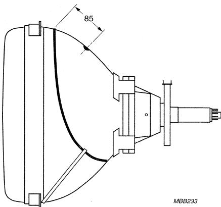
Fig.18 Position of the degaussing coil on the picture tube.
