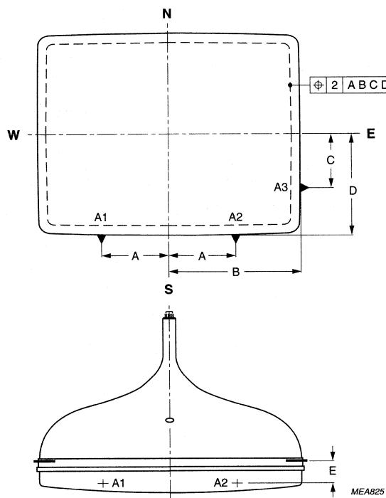
Fig.1 Phosphor alignment.
