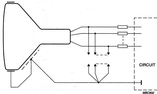
Fig.15 Flashover protection circuit.
