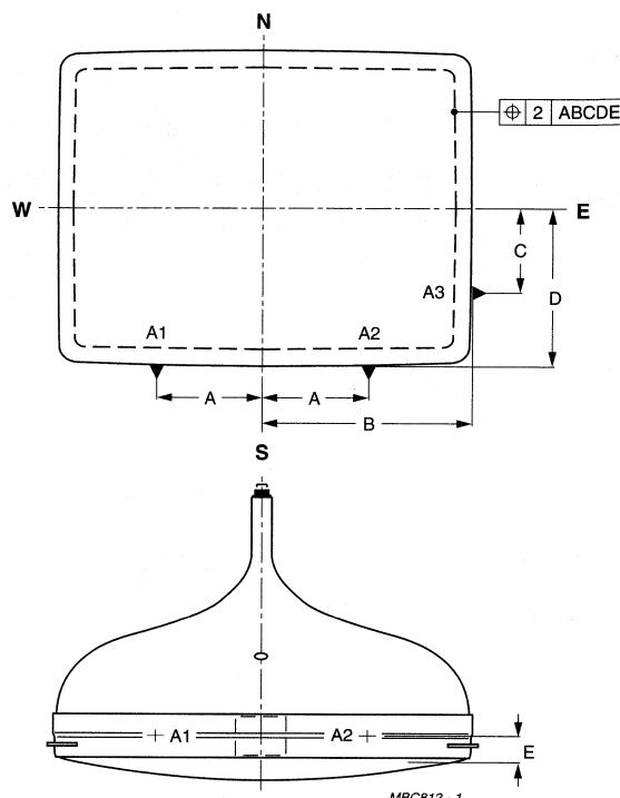
Fig.1 Phosphor alignment.
