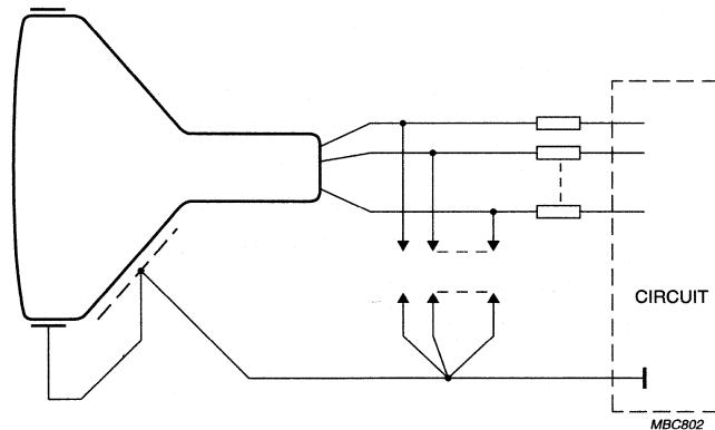
Fig.15 Flashover protection circuit.
