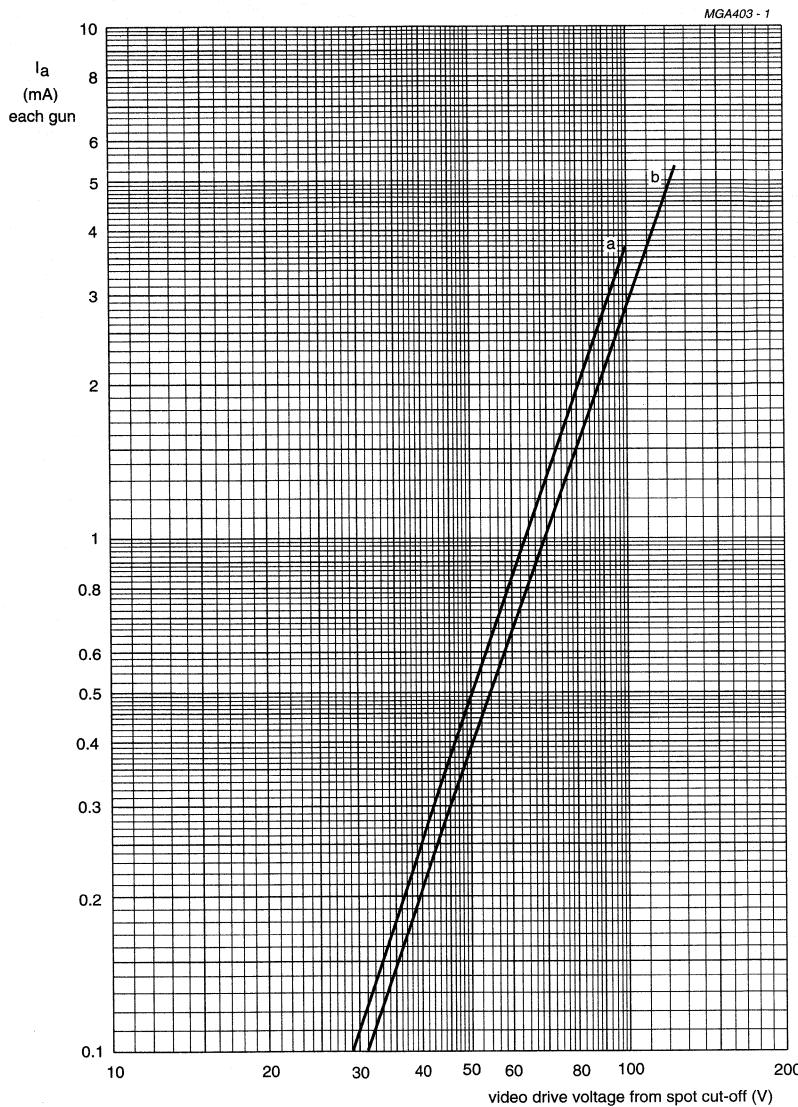
$V_f = 6.15 \text{ V}$ . $V_a = 23 \text{ kV}$ . $V_{g3}$  adjusted for focus.V<sub>g2</sub> (each gun) adjusted to provide spot cut-off for V<sub>k</sub> = 100 V (curve a) and V<sub>k</sub> = 125 V (curve b).
