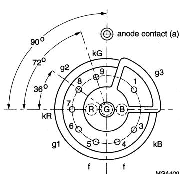
Fig.9 Pin arrangement.
