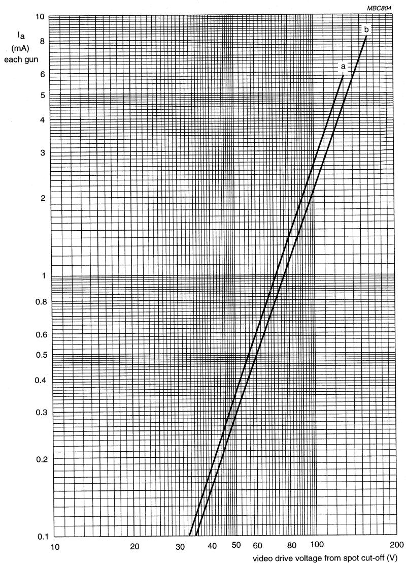
$V_f = 6.15 \text{ V}$ . $V_{a,g4} = 29.5 \text{ kV}$ . $V_{g3}$  adjusted for focus. $V_{g2}$  (each gun) adjusted to provide spot cut-off for  $V_k = 130 \text{ V}$  (curve a) and  $V_k = 160 \text{ V}$  (curve b).
