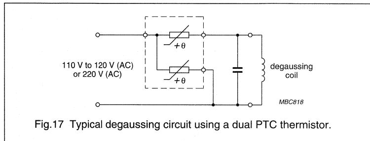
Fig.17 Typical degaussing circuit using a dual PTC thermistor.
