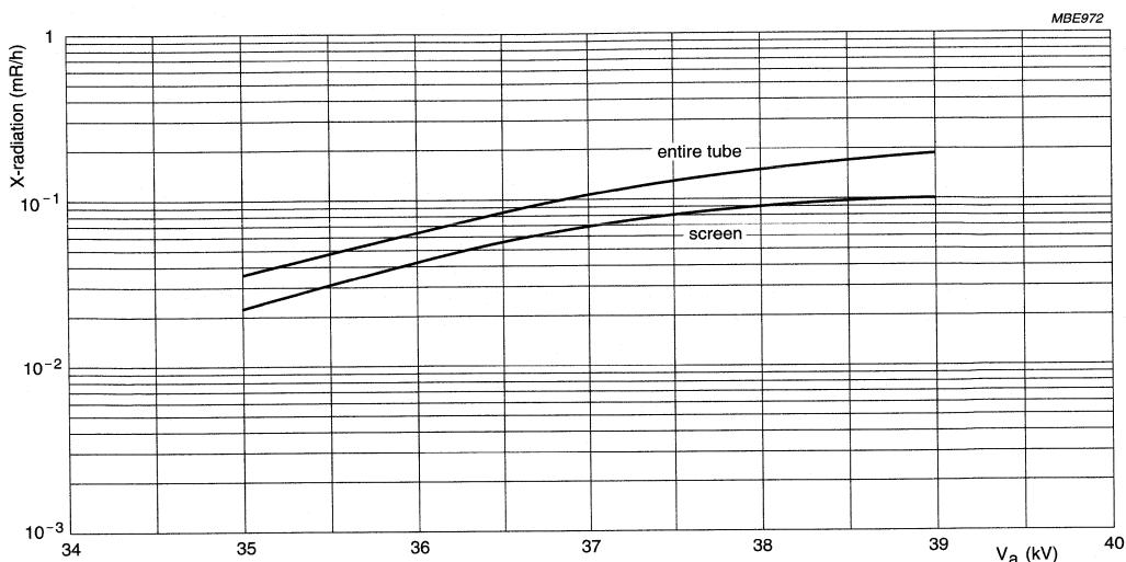
Fig.13 X-radiation limit curves at a constant anode current of 300  $\mu$ A.
