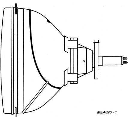
**Fig.19 Position of a single degaussing coil on the picture tube.**
