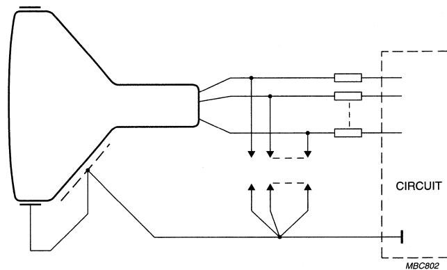
Fig.15 Flashover protection circuit.
