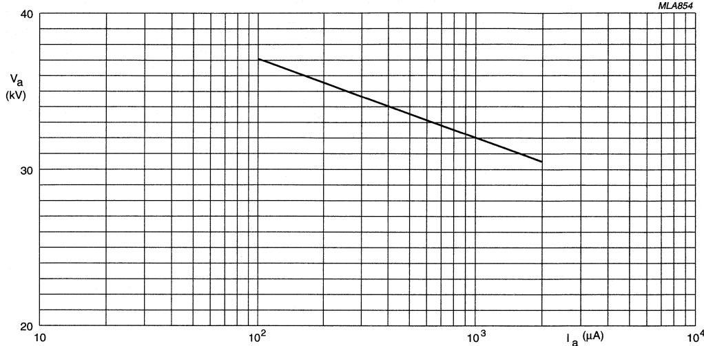
The X-radiation emitted will also not exceed 1  $\mu\text{Sv/h}$  for anode voltage and current combinations shown in the iso-exposure-rate limit curve.
