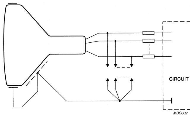
Fig.15 Flashover protection circuit.
