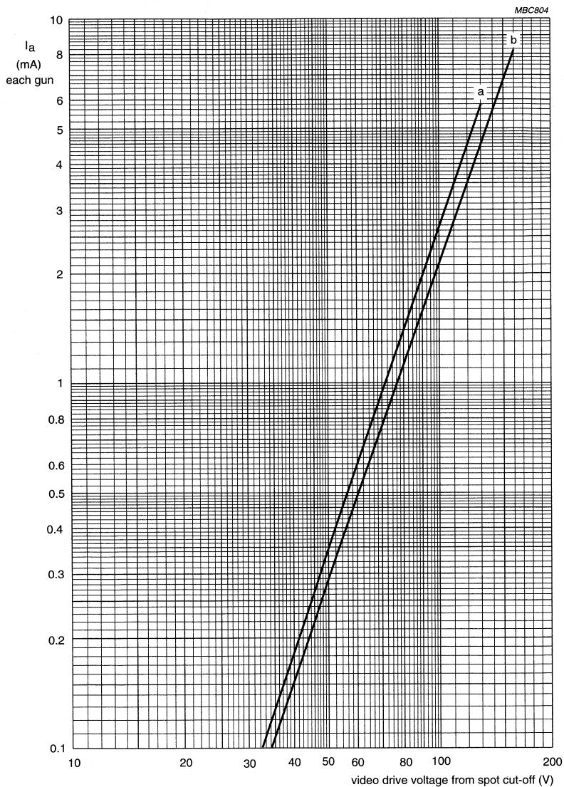
$V_f = 6.15$  V. $V_a = 30$  kV. $V_{g5a}$  and  $V_{g5b}$  adjusted for focus. $V_{g2}$  (each gun) adjusted to provide spot cut-off for  $V_k = 130$  V (curve a) and  $V_k = 160$  V (curve b).
