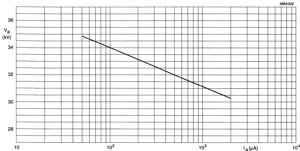
The X-radiation emitted will also not exceed 1  $\mu\text{Sv}/\text{h}$  for anode voltage and current combinations shown in the iso-exposure-rate limit curve.
