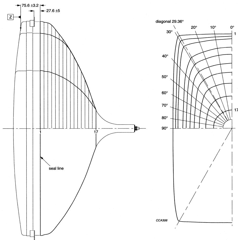
Fig.10 Maximum cone contour.
