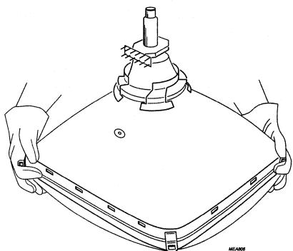
Fig.20 Lifting tube from face-down position.
