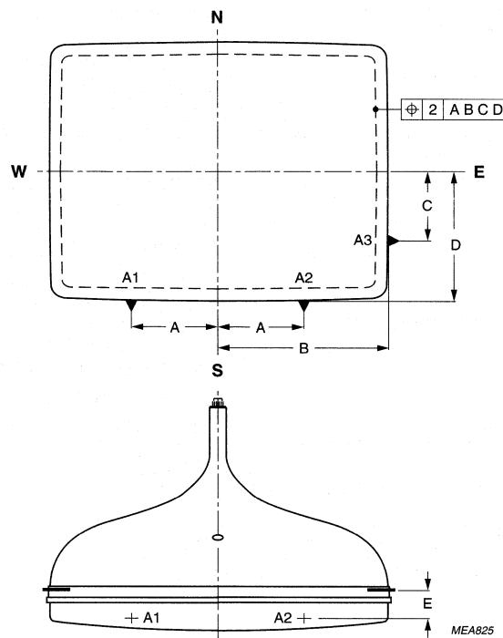
Fig.1 Phosphor alignment.
