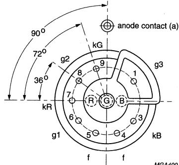
Fig.9 Pin arrangement.
