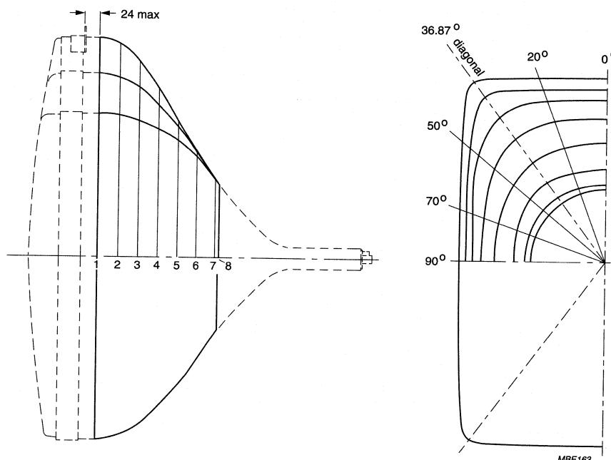
Fig.12 Maximum cone contour.
