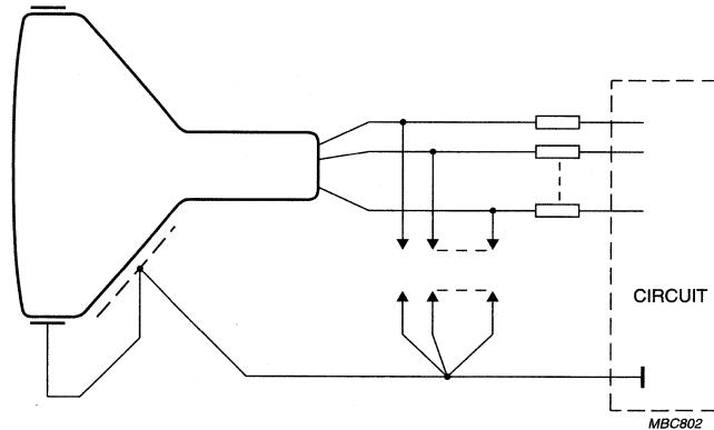
Fig.15 Flashover protection circuit.
