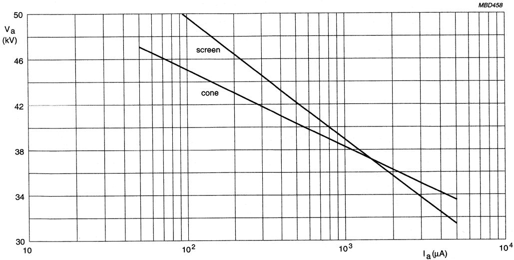
The tube does not emit X-radiation above 1  $\mu$ Sv/h when operated at 30 kV and 1.5 mA.
