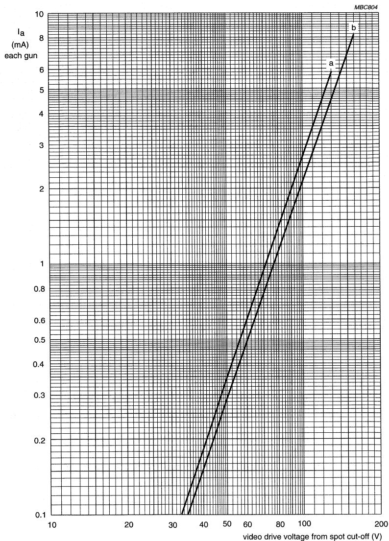
$V_f = 6.15 \text{ V.}$  $V_{a,g4} = 27.5 \text{ kV.}$  $V_{g3}$  adjusted for focus. $V_{g2}$  (each gun) adjusted to provide spot cut-off for  $V_k = 130 \text{ V}$  (curve a) and  $V_k = 160 \text{ V}$  (curve b).**Fig.14 Typical cathode drive characteristics.**
