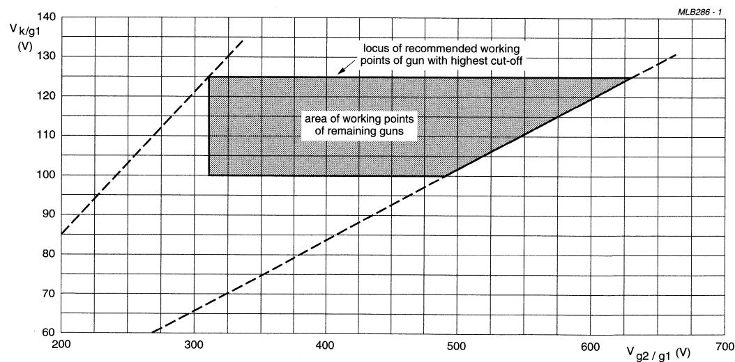
Grid 2 voltage ( $V_{g2}$ ) adjusted for highest gun spot cut-off voltage  $V_k = 125$  V.
