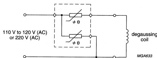
Fig.18 Typical degaussing circuit using dual PTC thermistor.
