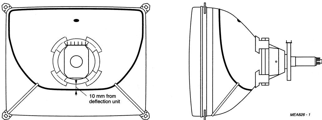
Fig.19 Position of a single degaussing coil on the picture tube.
