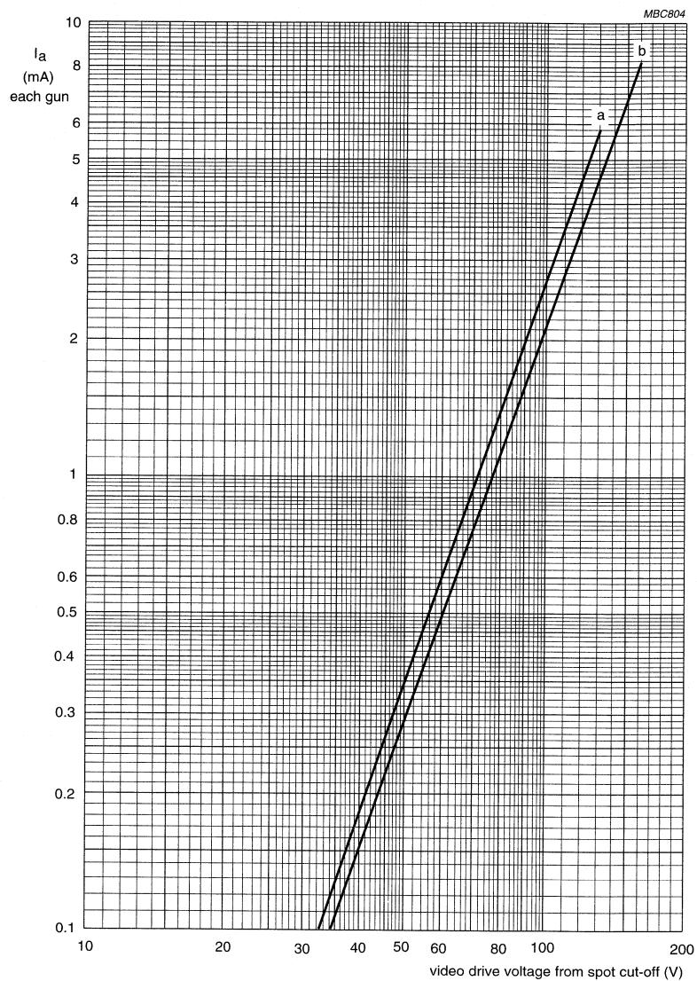
$V_f = 6.15$  V. $V_{a,g4} = 29.5$  kV. $V_{g3}$  adjusted for focus. $V_{g2}$  (each gun) adjusted to provide spot cut-off for  $V_k = 130$  V (curve a) and  $V_k = 160$  V (curve b).
