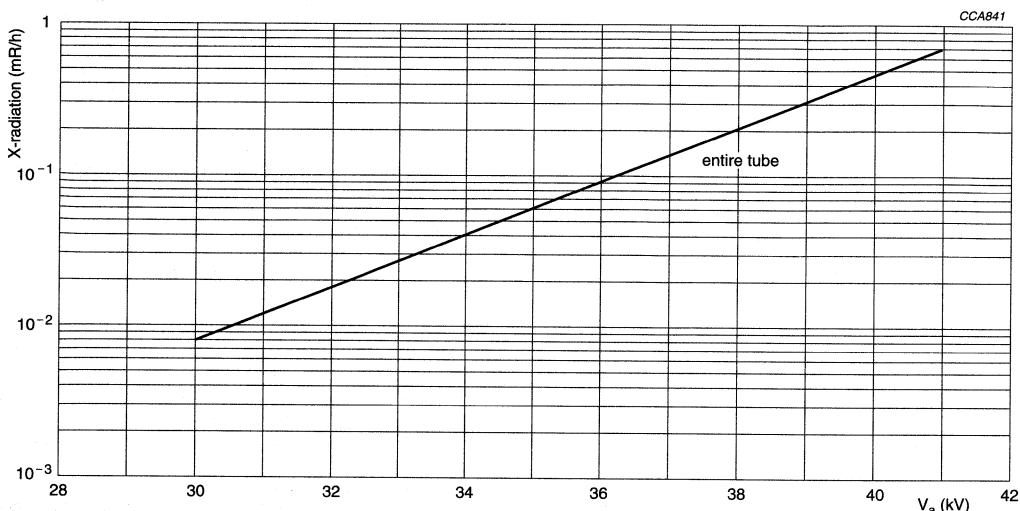
Fig.16 X-radiation limit curves at a constant anode current of 300  $\mu\text{A}$ .
