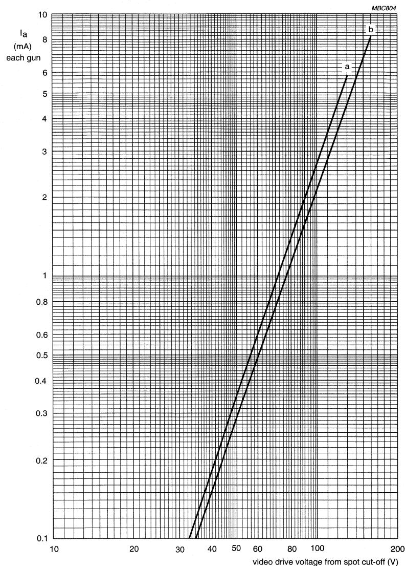
$V_f = 6.15$  V. $V_{a,g4} = 27.5$  kV. $V_{g3}$  adjusted for focus. $V_{g2}$  (each gun) adjusted to provide spot cut-off for  $V_k = 130$  V (curve a) and  $V_k = 160$  V (curve b).
