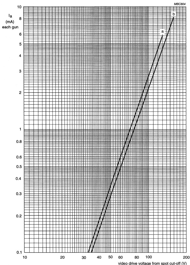
$V_f = 6.15 \text{ V}$ . $V_{a,g4} = 27.5 \text{ kV}$ . $V_{g3}$  adjusted for focus. $V_{g2}$  (each gun) adjusted to provide spot cut-off for  $V_k = 130 \text{ V}$  (curve a) and  $V_k = 160 \text{ V}$  (curve b).
