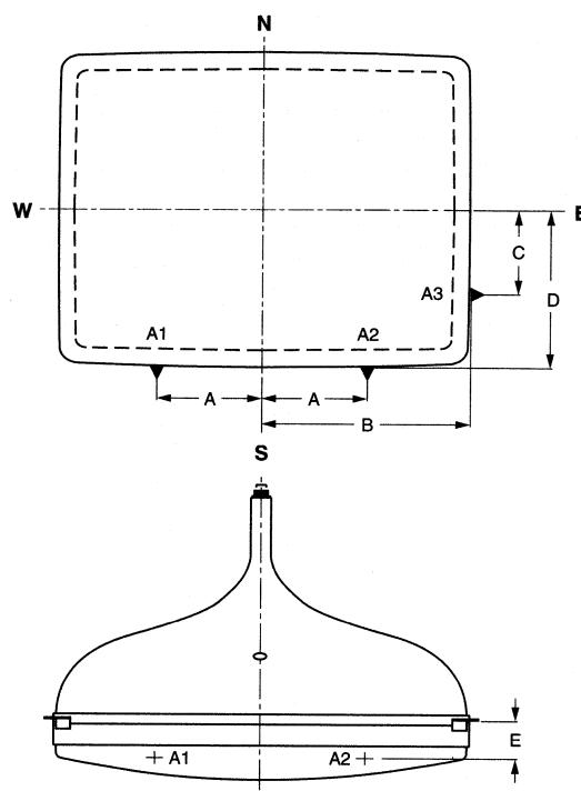
Fig.1 Phosphor alignment.
