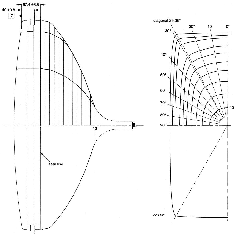
Fig.11 Maximum cone contour.
