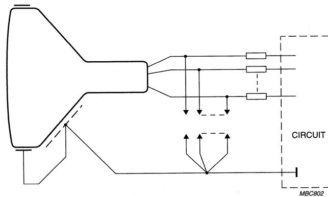
Fig.12 Flashover protection circuit.
