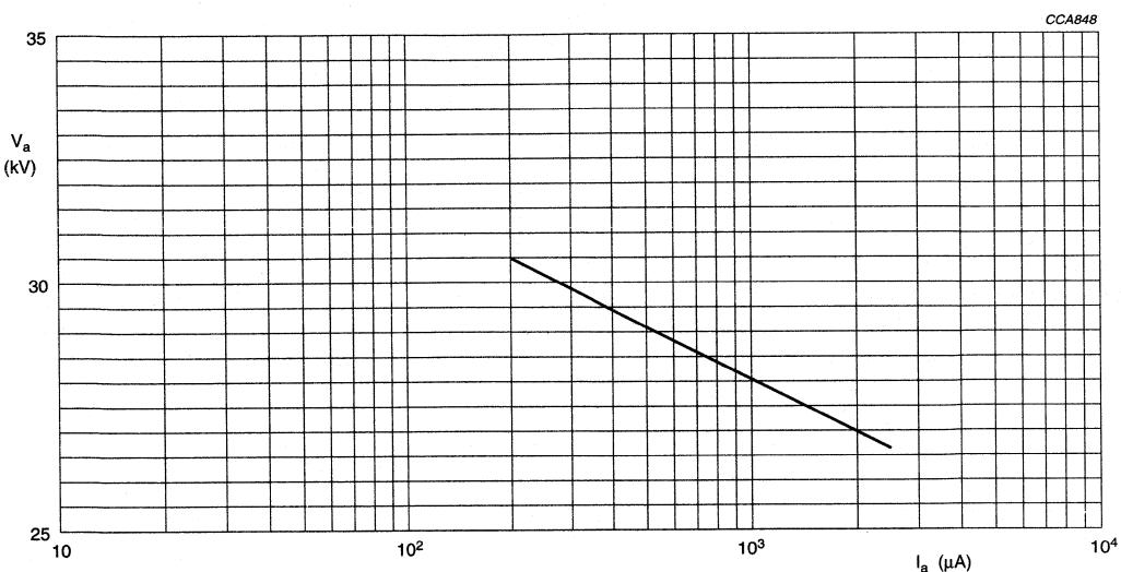
The tube does not emit X-radiation above 1  $\mu\text{Sv}/\text{h}$  when operated at 33 kV and 1.8 mA. The X-radiation emitted will also not exceed 1  $\mu\text{Sv}/\text{h}$  for anode voltage and current combinations shown in the iso-exposure-rate limit curve.
