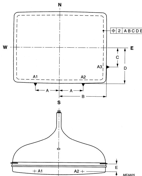
Fig.1 Phosphor alignment.
