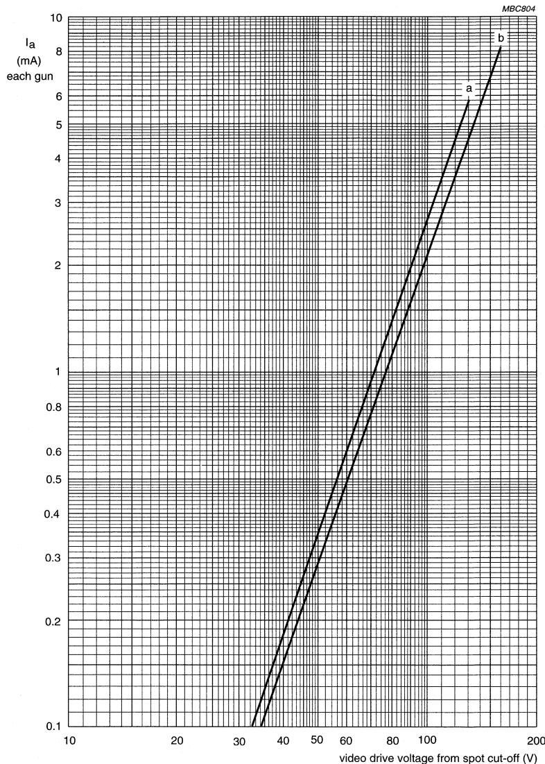
$V_f = 6.15 \text{ V}$ . $V_a = 30 \text{ kV}$ . $V_{g3}$  adjusted for focus. $V_{g2}$  (each gun) adjusted to provide spot cut-off for  $V_k = 130 \text{ V}$  (curve a) and  $V_k = 160 \text{ V}$  (curve b).
