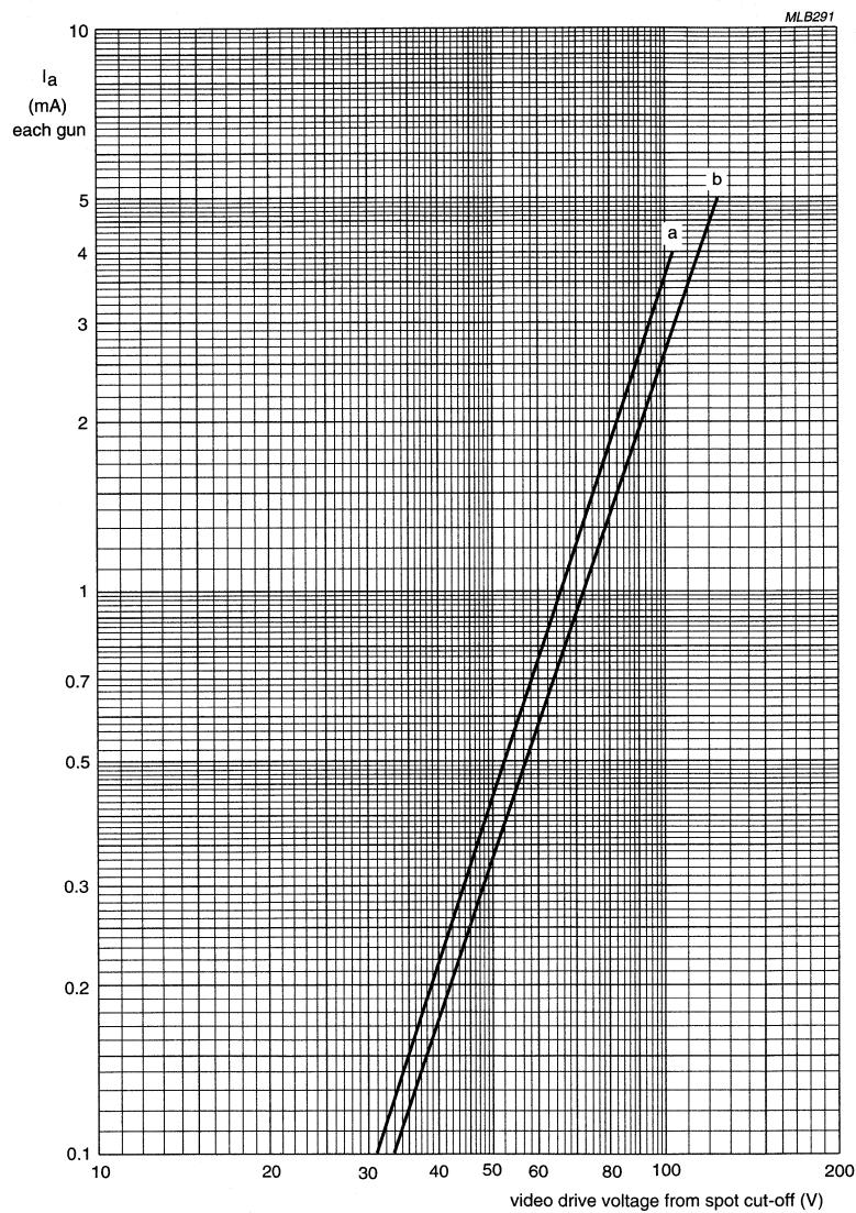
$V_f = 6.15$  V. $V_{a,g4} = 25$  kV. $V_{g2}$  adjusted for focus. $V_{g2}$  (each gun) adjusted to provide spot cut-off for  $V_k = 105$  V (curve a) and  $V_k = 130$  V (curve b).
