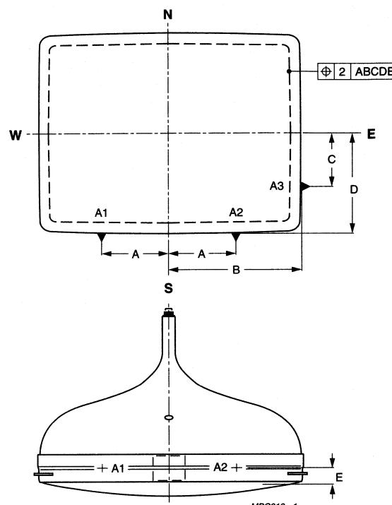
Fig.1 Phosphor alignment.
