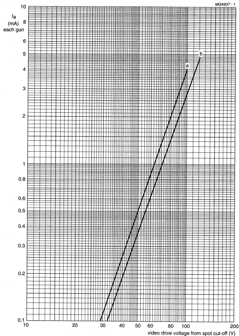
$V_f = 6.15 \text{ V.}$  $V_{a,g4} = 23 \text{ kV.}$  $V_{g3}$  adjusted for focus. $V_{g2}$  (each gun) adjusted to provide spot cut-off for  $V_k = 100 \text{ V}$  (curve a),  $V_k = 125 \text{ V}$  (curve b).
