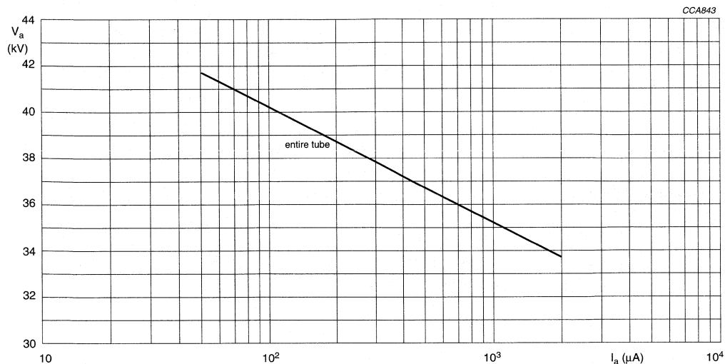
The tube does not emit X-radiation above  $1 \mu\text{Sv}/\text{h}$  when operated at 33 kV and 1.8 mA. The X-radiation emitted will also not exceed  $1 \mu\text{Sv}/\text{h}$  for anode voltage and current combinations shown in the iso-exposure-rate limit curve.
