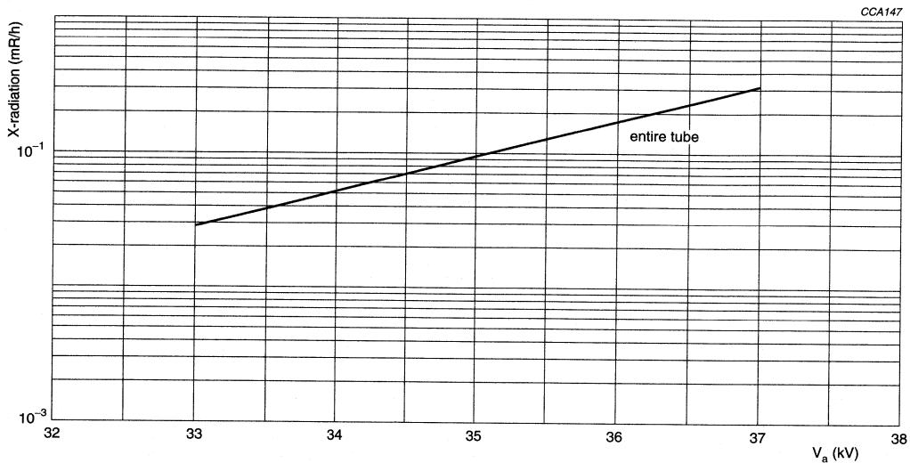
Fig.15 X-radiation limit curves at a constant anode current of 300  $\mu$ A.
