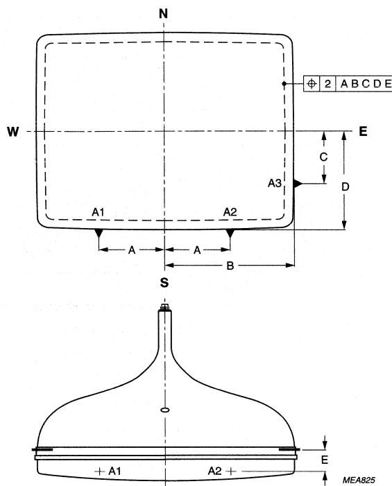
Fig.1 Phosphor alignment.
