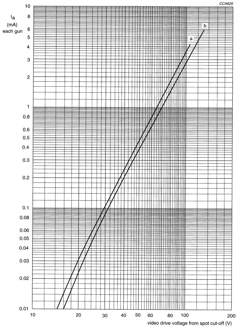
$V_f = 6.15$  V. $V_a = 25$  kV. $V_{g3}$  adjusted for focus. $V_{g2}$  (each gun) adjusted to provide spot cut-off for  $V_k = 105$  V (curve a) and  $V_k = 130$  V (curve b).
