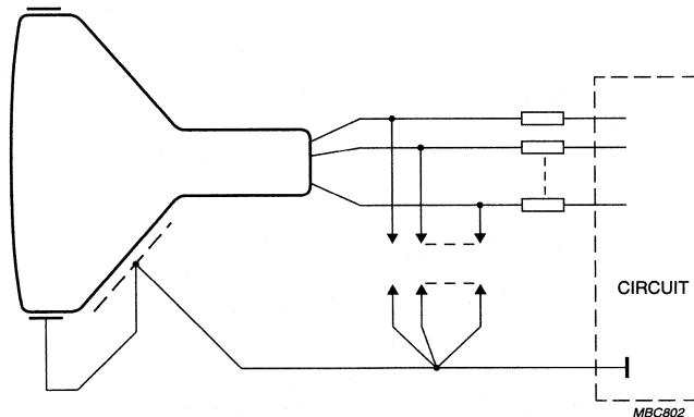
Fig.15 Flashover protection circuit.
