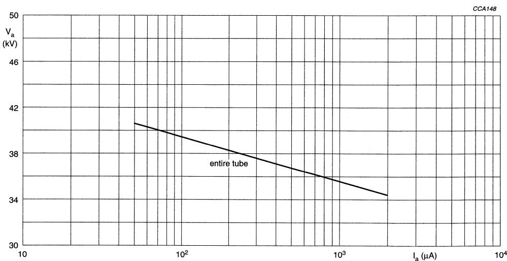
Fig.16 Iso-exposure-rate limit curves at 0.5 mR/h.
