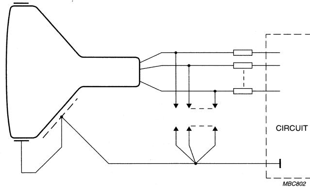
Fig.15 Flashover protection circuit.
