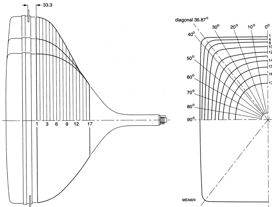
**Fig.12 Maximum cone contour.**
