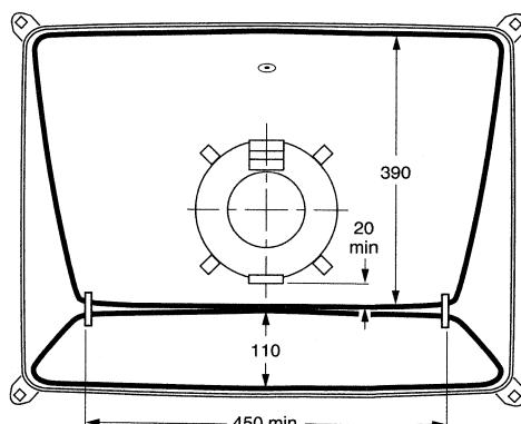
Fig.20 Mounting of degaussing coils on the picture tube.
