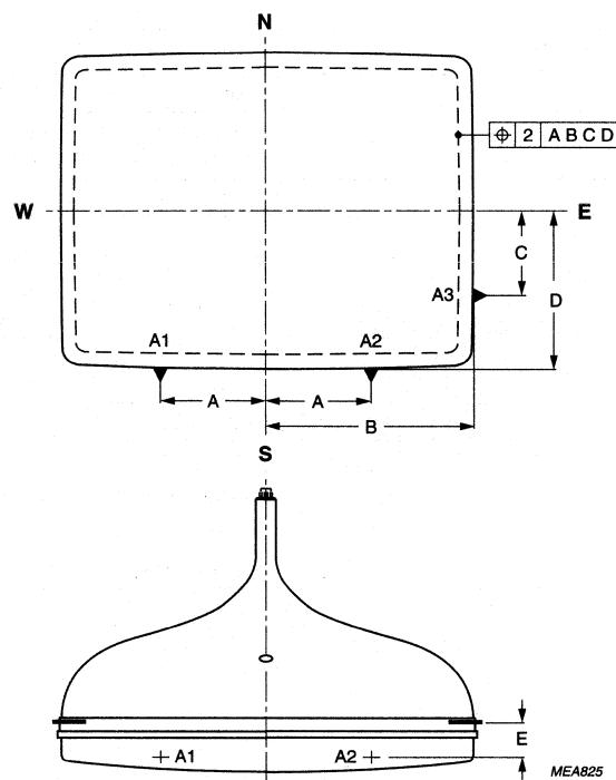
Fig.1 Phosphor alignment.
