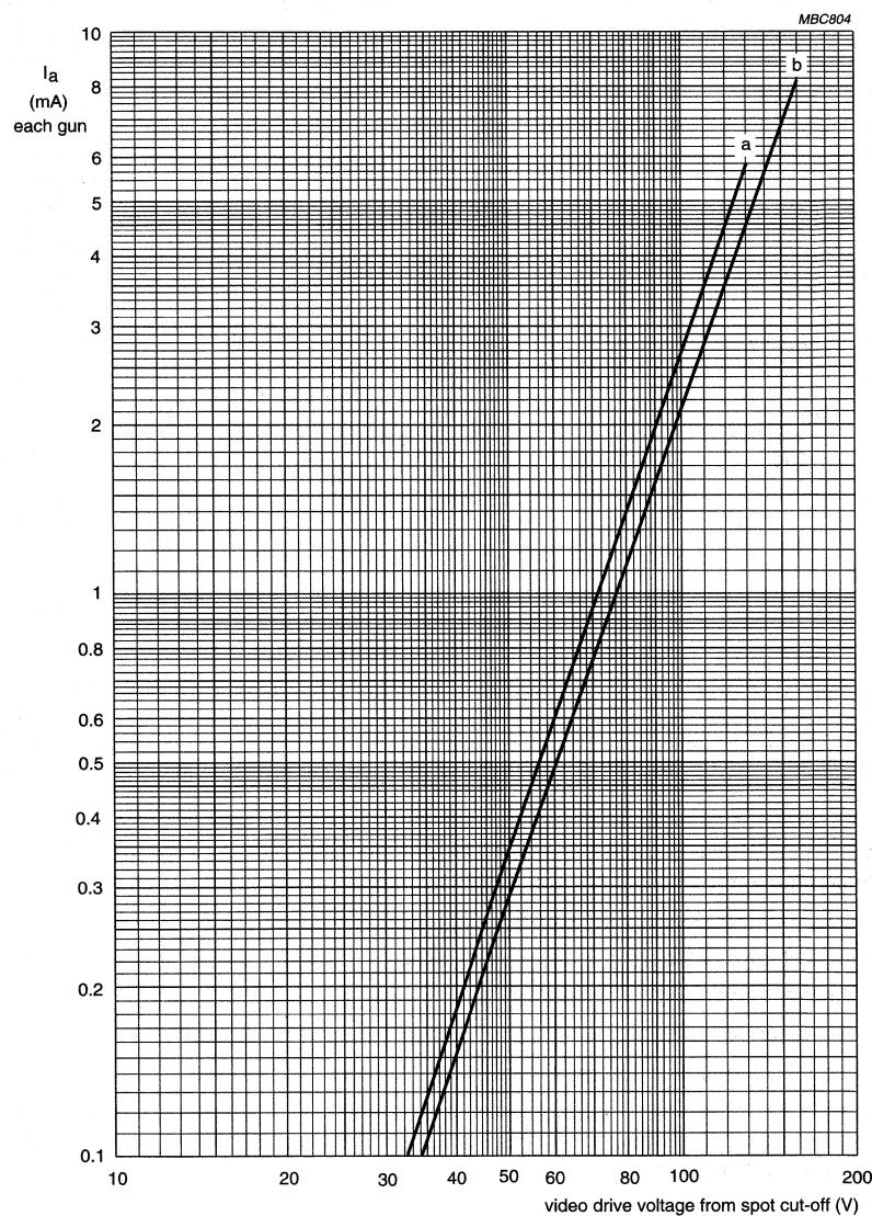
$V_f = 6.15$  V. $V_{a,q4} = 27.5$  kV. $V_{g3}$  adjusted for focus. $V_{g2}$  (each gun) adjusted to provide spot cut-off for  $V_k = 130$  V (curve a) and  $V_k = 160$  V (curve b).
