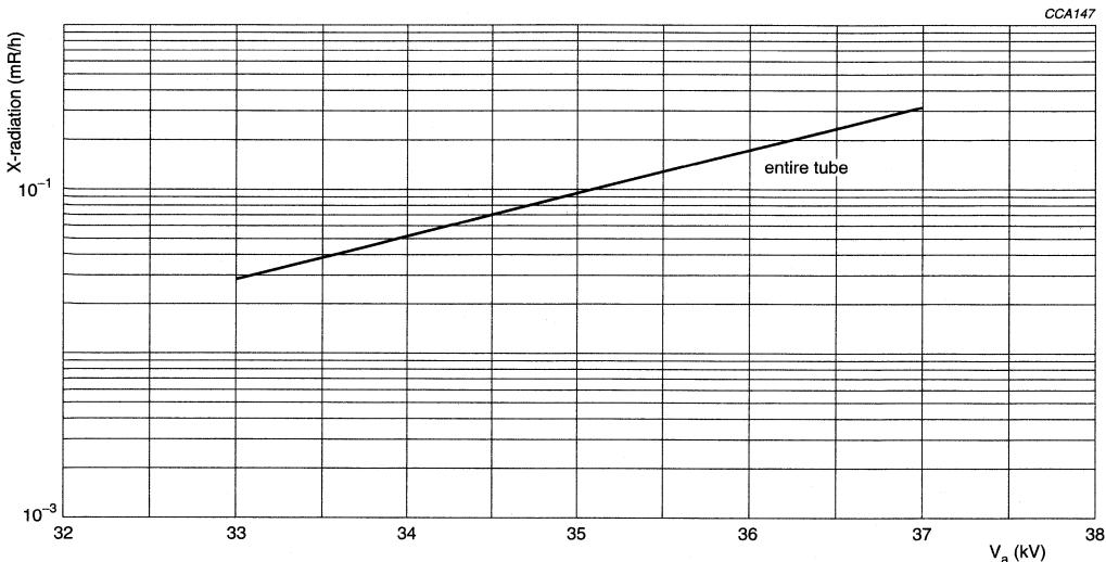
Fig.15 X-radiation limit curves at a constant anode current of 300  $\mu$ A.
