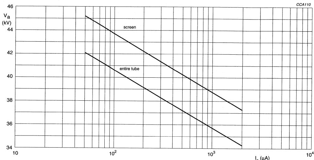
The tube does not emit X-radiation above 1  $\mu\text{Sv}/\text{h}$  when operated at 33 kV and 2.0 mA. The X-radiation emitted will also not exceed 1  $\mu\text{Sv}/\text{h}$  for anode voltage and current combinations shown in the iso-exposure-rate limit curve.
