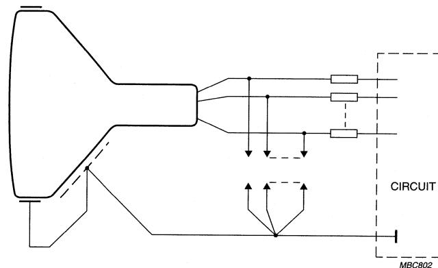
Fig.14 Flashover protection circuit.
