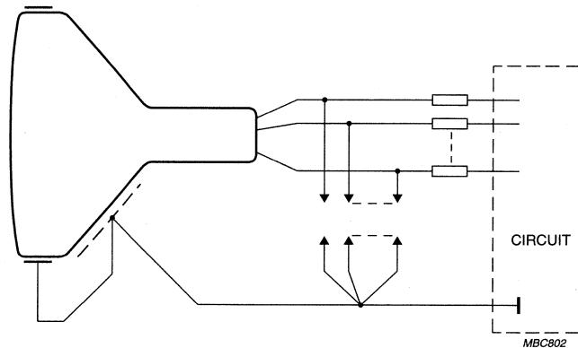
Fig.14 Flashover protection circuit.
