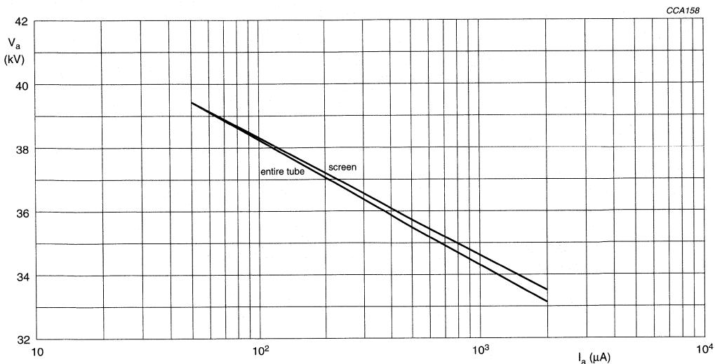
The tube does not emit X-radiation above 1  $\mu\text{Sv/h}$  when operated at 33 kV and 1.8 mA. The X-radiation emitted will also not exceed 1  $\mu\text{Sv/h}$  for anode voltage and current combinations shown in the iso-exposure-rate limit curve.
