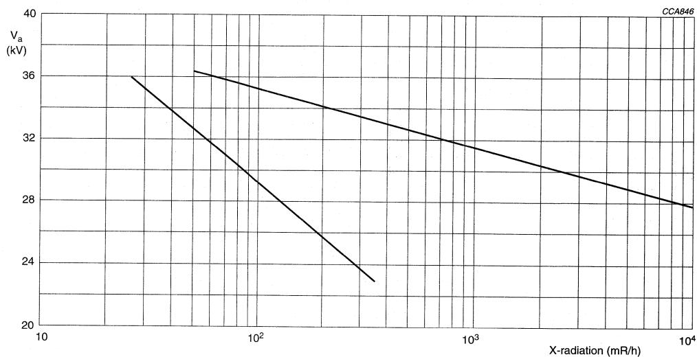
Fig.15 Iso-exposure-rate limit curves at 0.5 mR/h.
