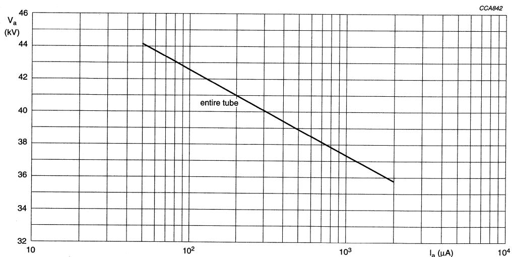
Fig.17 Iso-exposure-rate limit curves at 0.5 mR/h.
