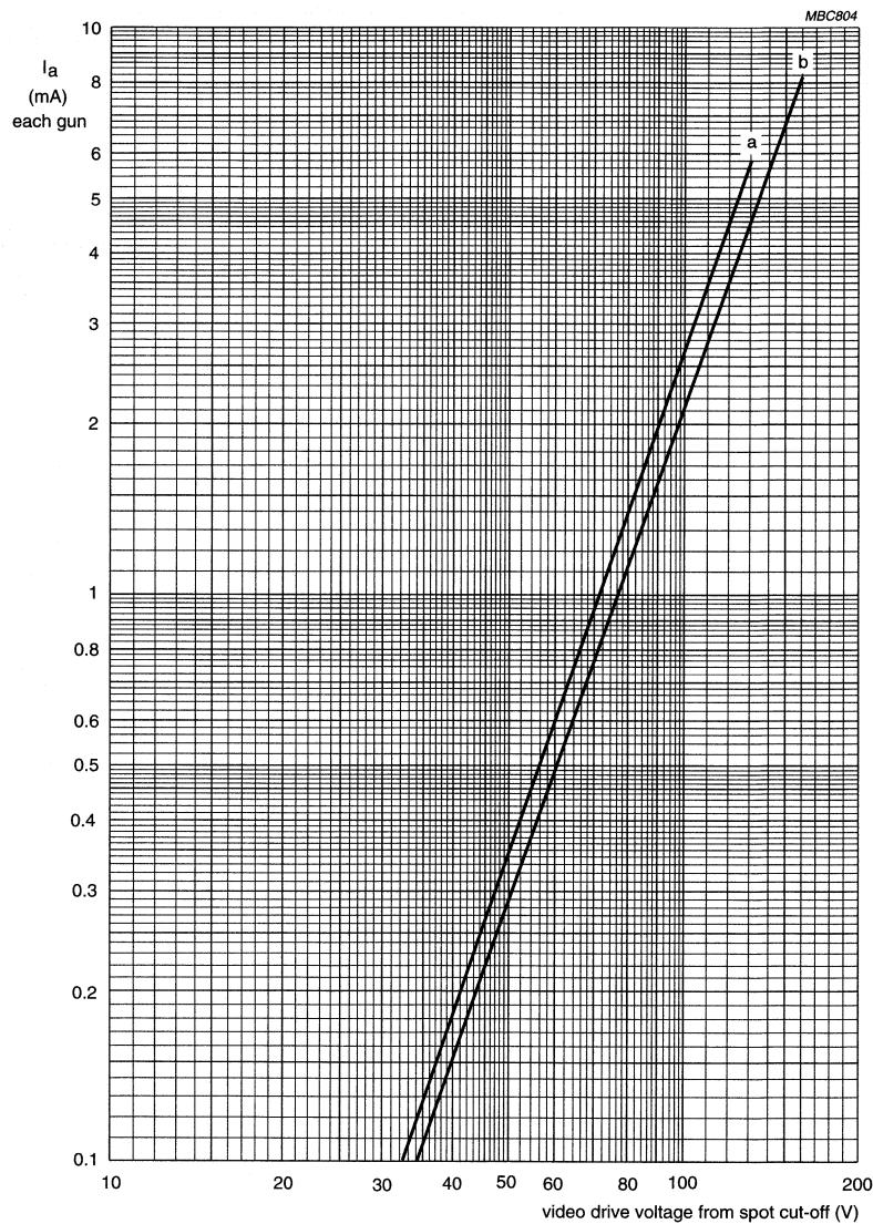
Fig.13 Typical cathode drive characteristics.
