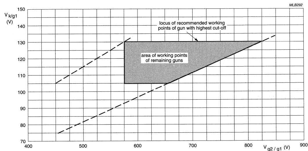
Grid 2 voltage ( $V_{g2}$ ) adjusted for highest gun spot cut-off voltage  $V_k = 130$  V.
