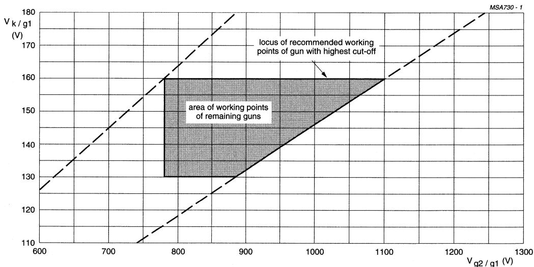
Grid 2 voltage ( $V_{g2}$ ) adjusted for highest gun spot cut-off voltage  $V_k = 160$  V.
