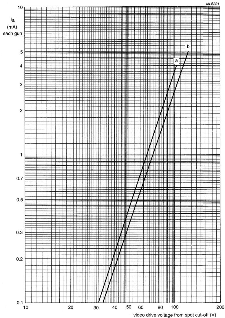
$V_f = 6.15$  V. $V_{a,g4} = 25$  kV. $V_{g3}$  adjusted for focus. $V_{g2}$  (each gun) adjusted to provide spot cut-off for  $V_k = 105$  V (curve a) and  $V_k = 130$  V (curve b).
